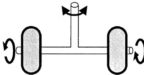
Fig. 2 –(B) The multiple dual active caster mechanisms.
