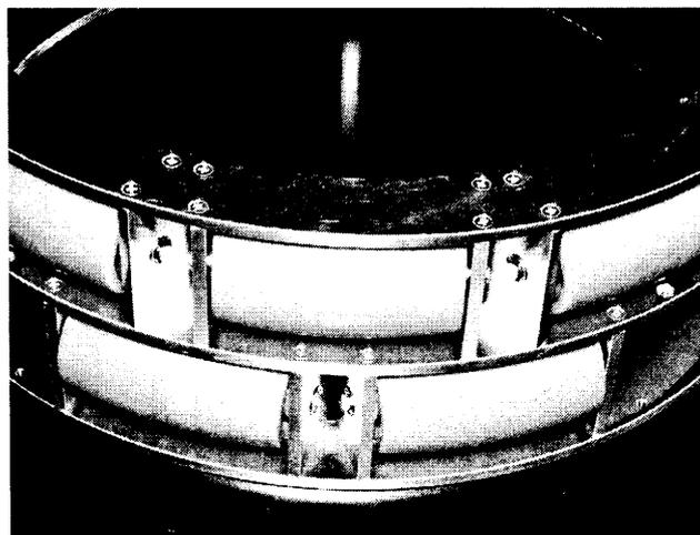
Fig. 4 The rear wheel of the wheelchair using dual-row omni wheel.
