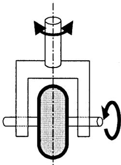
Fig. 2 –(A) The multiple active caster mechanisms.
