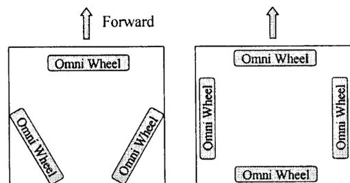
Fig. 1 - (B) Arrangements of the omni-wheels for omni-directional mobile robots.
