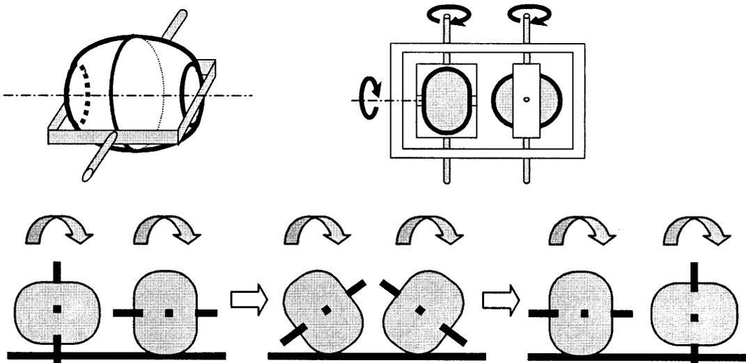
Fig. 3 Orthogonal Wheel Mechanism.
