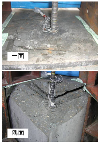
Fig. 9 Failure of Concrete Fig. 10 Failure of Bonded Anchor bars
