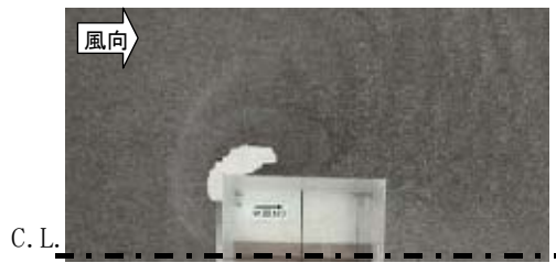
Photo2 Distribution of sand erosion/deposition around the cube after 5min.
