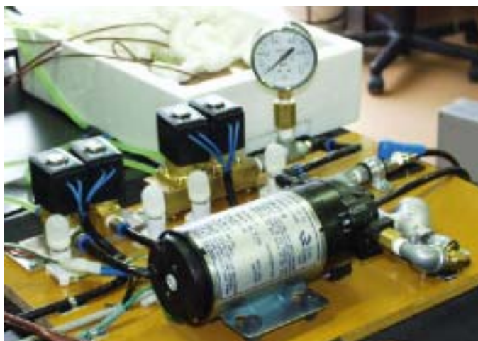
Fig. 5 Water-supply system (feed pump and solenoid valves).
