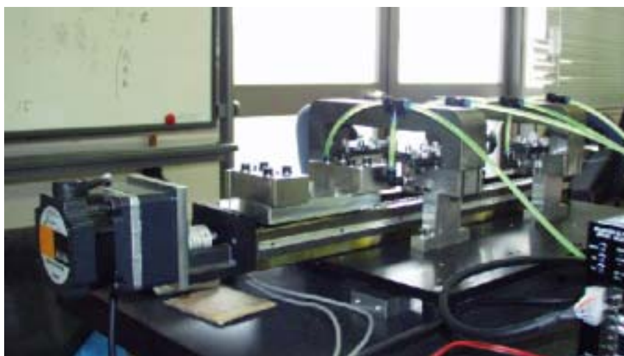
Fig.2 Overview of the reciprocal magnetic refrigerator.
