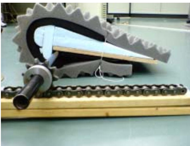
Fig. 4 Shape of abdomen - chest cushion and Sprocket & chain mechanism.
