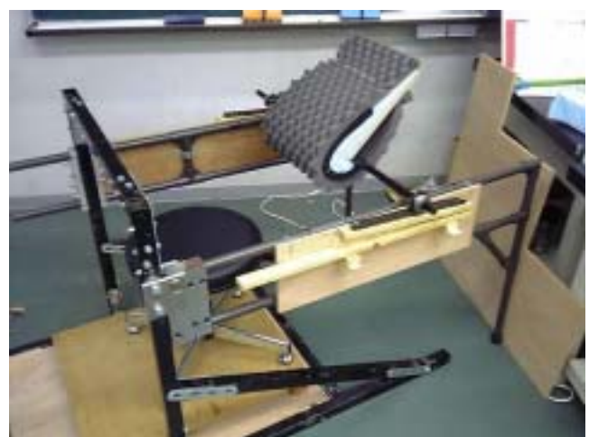
Fig.5 Assistive implement for changing clothes - Second type.
