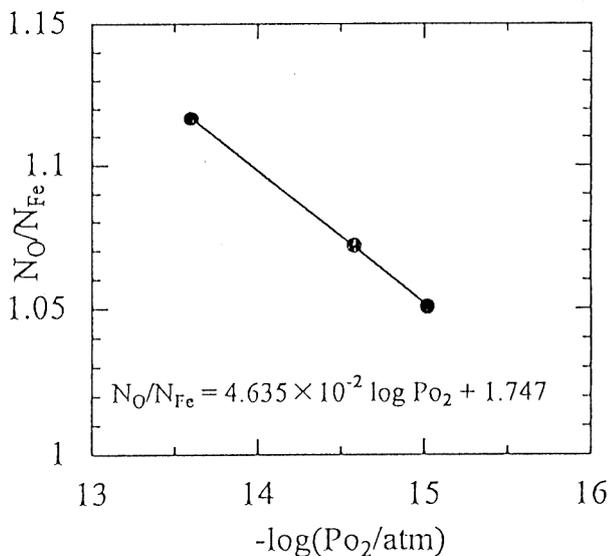
Fig. 1c. The relationship between the oxygen partial pressure,  $\log(P_{\text{O}_2}/\text{atm})$  and  $N_{\text{O}}/N_{\text{Fe}}$  in the FeO solid solution.
