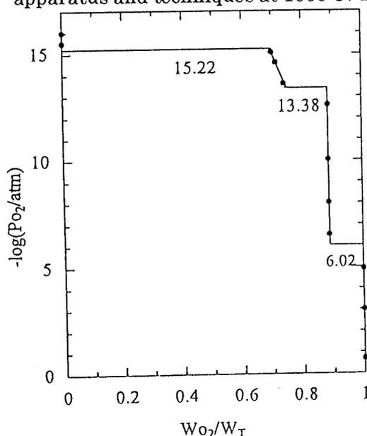
Fig. 1a. The relationship between the oxygen partial pressure,  $\log(P_{\text{O}_2}/\text{atm})$  and the weight change of samples,  $W_{\text{O}_2}/W_T$  in the Fe-O system.
