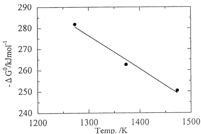
Fig. 4 The relationship between  $\Delta G^0$  for reaction 4) and the temperature.
