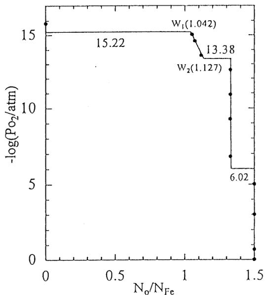
Fig. 1b. The relationship between the oxygen partial pressure,  $\log(P_{\text{O}_2}/\text{atm})$ , and the  $N_{\text{O}}/N_{\text{Fe}}$  mole fraction ratio in the Fe-O system.
