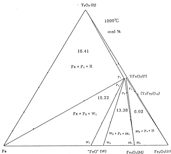
Fig. 3. Phase equilibrium in the  $Y_2O_3$ -Fe- $Fe_2O_3$  system at  $1000^\circ C$ . Numerical values indicated in the three phase regions are the oxygen partial pressures in  $-\log(P_{O_2}/atm)$  in equilibrium with the solid phases shown in each region. Abbreviations are the same as those in Table 2.
