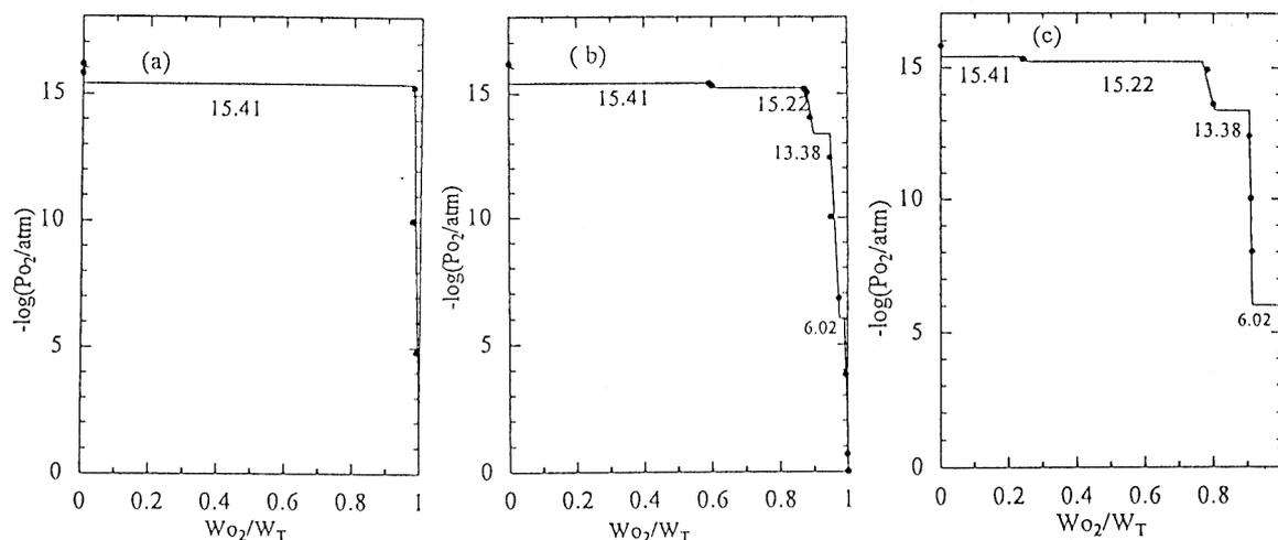
Fig. 2. The relationship between the oxygen partial pressure,  $\log(P_{O_2}/\text{atm})$ , and the weight change of the samples,  $W_{O_2}/W_T$ . (a)  $Y_2O_3/Fe_2O_3 = 0.6/0.4$ , (b)  $Y_2O_3/Fe_2O_3 = 0.4/0.6$ , and (c)  $Y_2O_3/Fe_2O_3 = 0.2/0.8$ .
